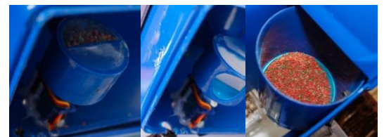
Fig. 5. Inside view of the fish feeder's actual prototype
