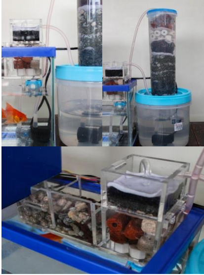
Fig. 6. Filter for the aquarium and water changer mechanism
